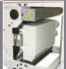
Combined UV chill drum hot air
